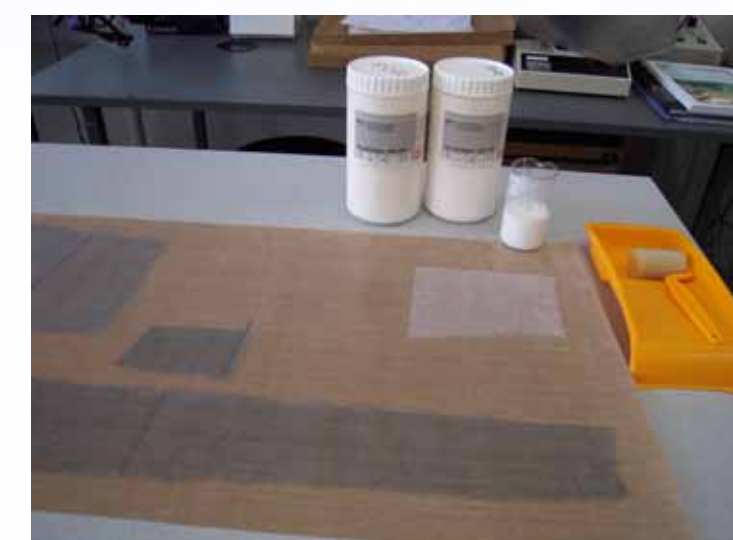
Fig. 1 Pasting the glue onto the netting on Teflon fabric. Mixture of thermoplastic acrylic Lascau 360: Lascau 498: water (1:1:5) was used as glue.
