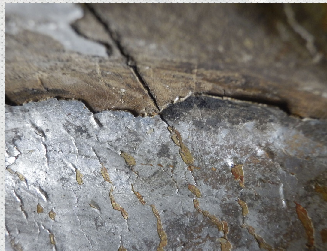
ill. 6. Flaking decor layers. Gilding is visible under the layer of aluminium covering.
